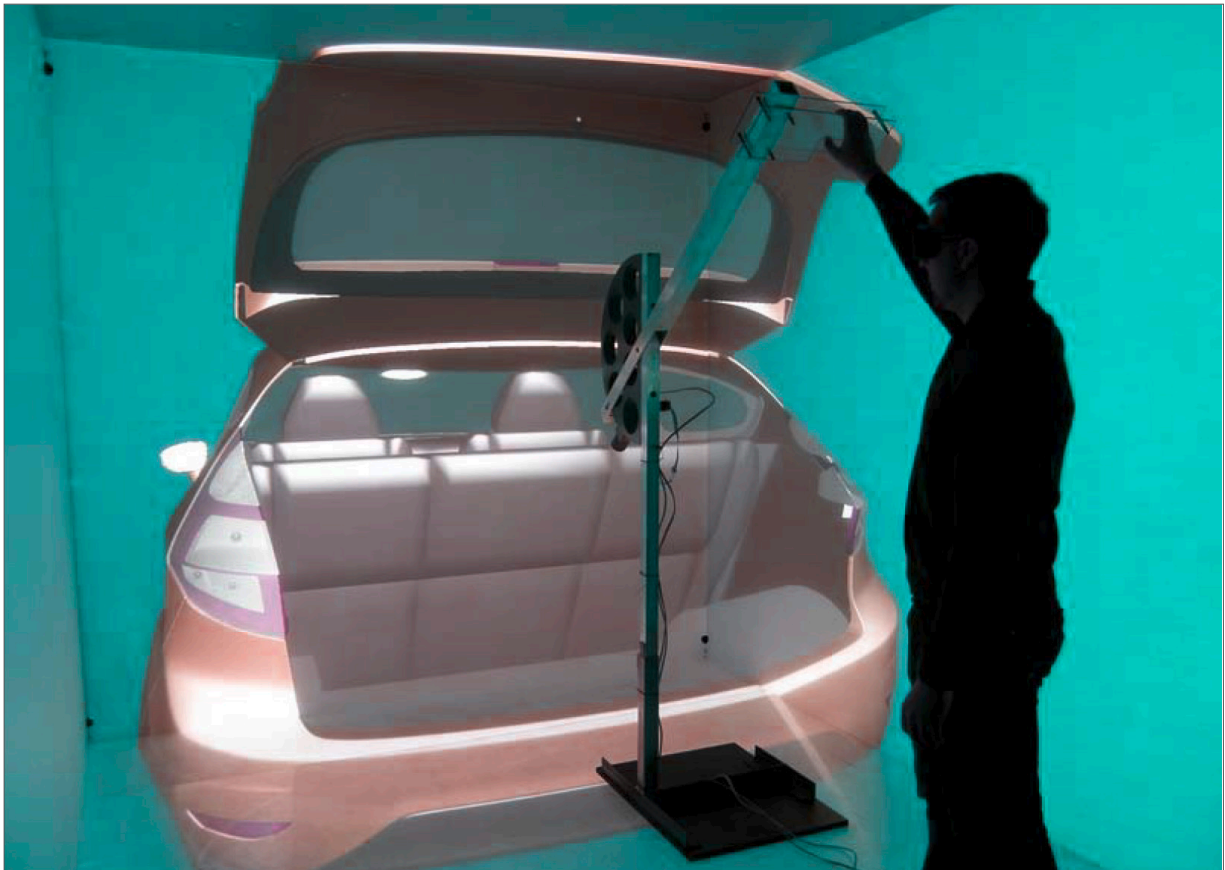
Figure 10: current use case 4 – SHP – example of SHP test of back door (right, (Beckmann-Dobrev et al. 2010, p 7))
