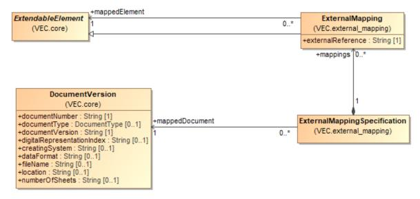
Figure 74: External Mapping
