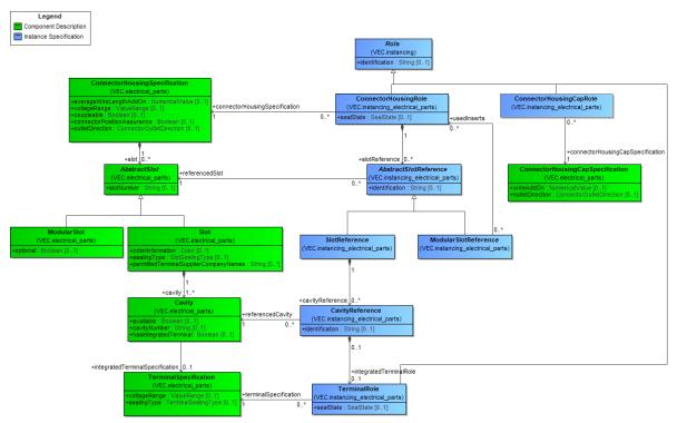
Figure 42: Instances of Connector Housings
