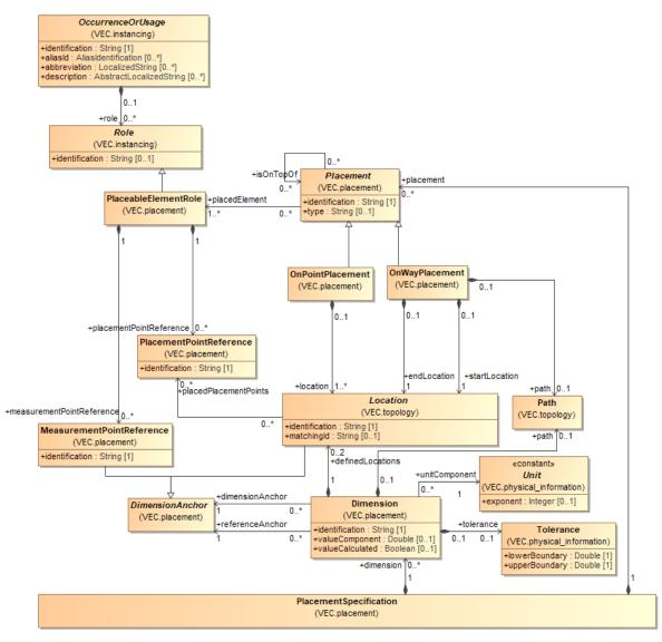
Figure 63: Placement and Dimensions
