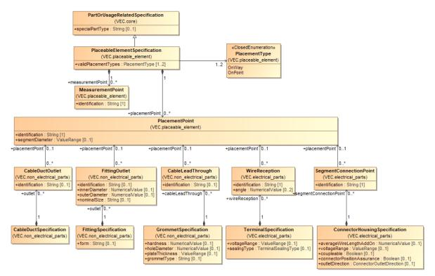
Figure 21: Placeable Elements
