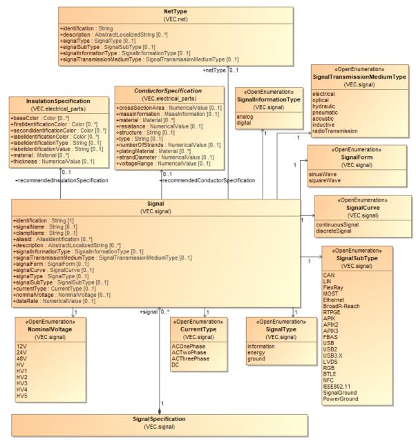
**Figure 66: Signal Specification**
