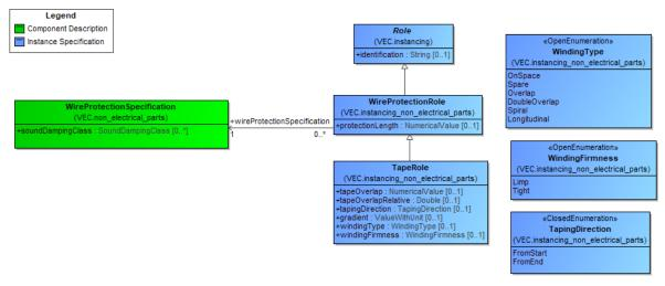
Figure 45: Instances of Wire Protections
