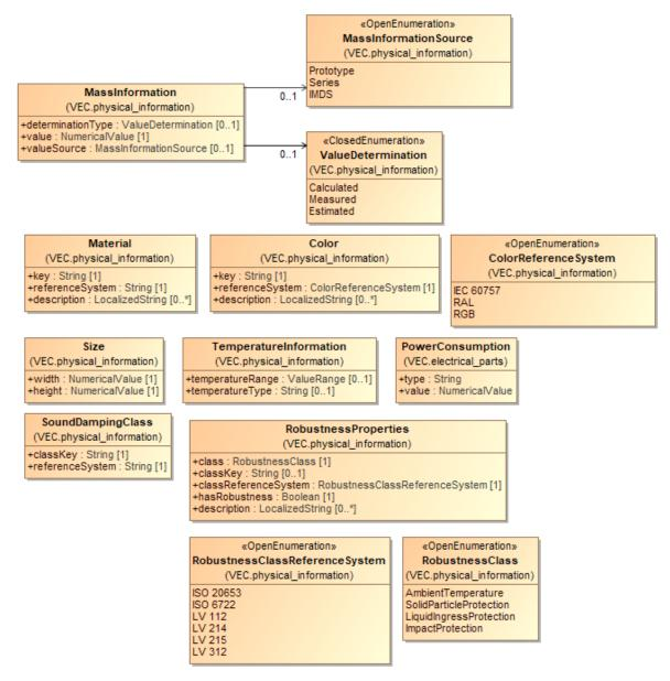
Figure 10: Foundation Classes for Physical Properties
