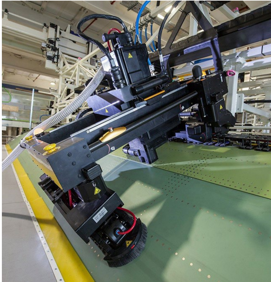
Figure 9: Light Flextrack drilling robot system (MTM Robotics)
